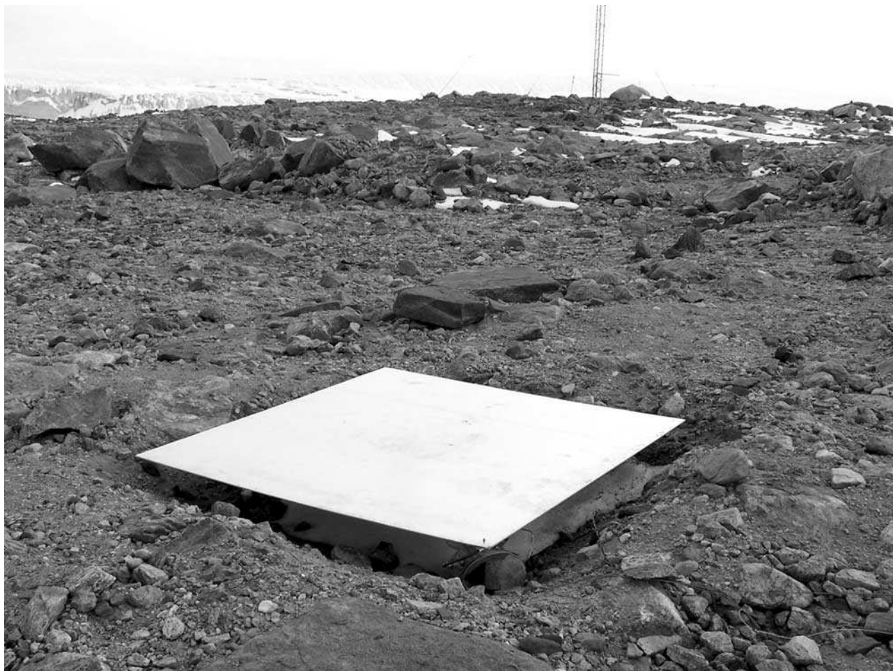
Figure 2. Air-Earth current plate antenna installed at Maitri.
