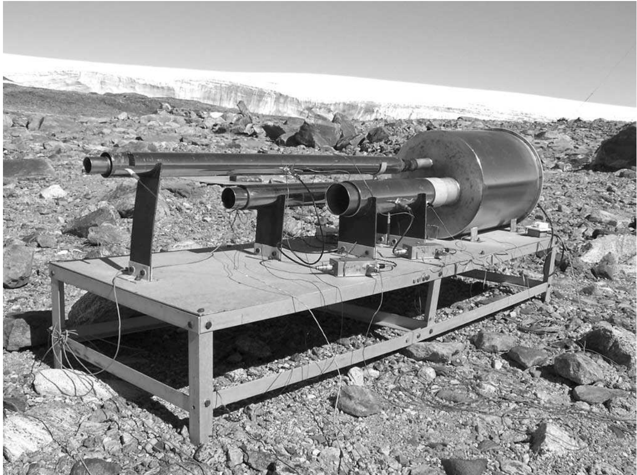
Figure 1. Ion counter installed at Maitri.
