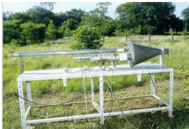
Atmospheric Ion counter at the Atmospheric Electricity Observatory
