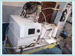
Installation of Scanning Mobility Particle Sizer (SMPS) onboard the aircraft during ICARB
