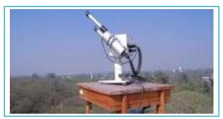
An automatic sun tracking sun/sky radiometer (Prede Model POM-01L) has been installed at the IITM New Delhi Branch on 17th February 2006 to monitor aerosol optical properties at the urban location under the ICARB Campaign.
