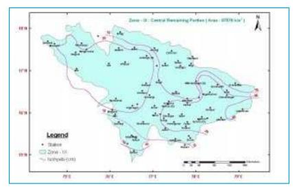
*Fig. 20 : Transposed Isohyetal map of 21-23 Sept., 1949 (3-day) rainstorm over Zone – IX of the Krishna basin.*
