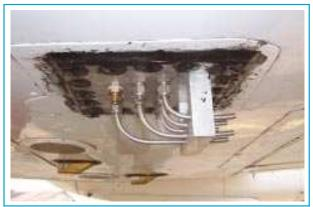
The air inlet tube installed beneath the Beachcraft aircraft
