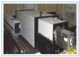
Laser Raman Spectrometer has been installed at the Institute in November 2005. It is a double monochrometer spectrometer. Argon ion laser is used as source. It will operate at two wavelengths 514.5 nm in green region and 488.0 nm in blue region. This system will be used to investigate the molecules present in a particular sample and chemical composition of aerosols collected from different atmospheric conditions.
