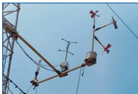
Experimental set-up at NCAOR, Goa using Sonic anemometer and \text{CO}_2 / \text{H}_2\text{O} analyzer systems during ARMEX Phase II
