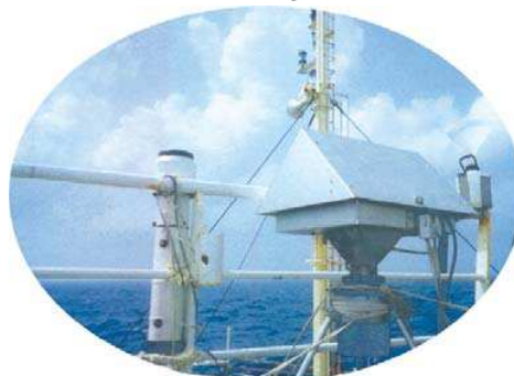
Aerosol sampling using high volume air sampler over the Arabian Sea onboard ORV Sagar Kanya during ARMEX
