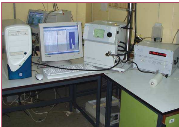
Scanning mobility particle sizer (upper) and Aerodynamic particle sizer (lower) installed onboard ORV Sagar Kanya during Pilot Expedition to Southern Ocean
