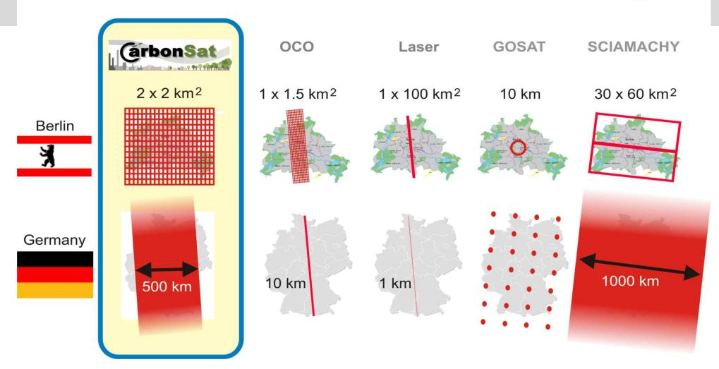
CarbonSat enables new important application areas: CO<sub>2</sub> and CH<sub>4</sub> emission "hot spot" detection and monitoring (power plants, …)
