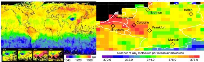
Global CO<sub>2</sub> and CH<sub>4</sub> measurement from SCIAMACHY on ENVISAT
