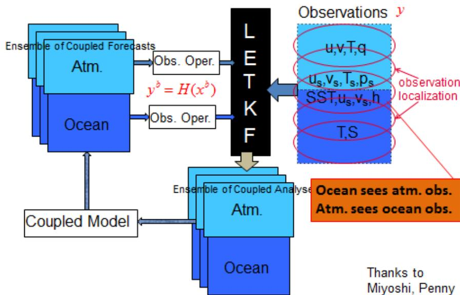
**Fig. 13:** Schematic figure for Strongly coupled LETKF assimilation
