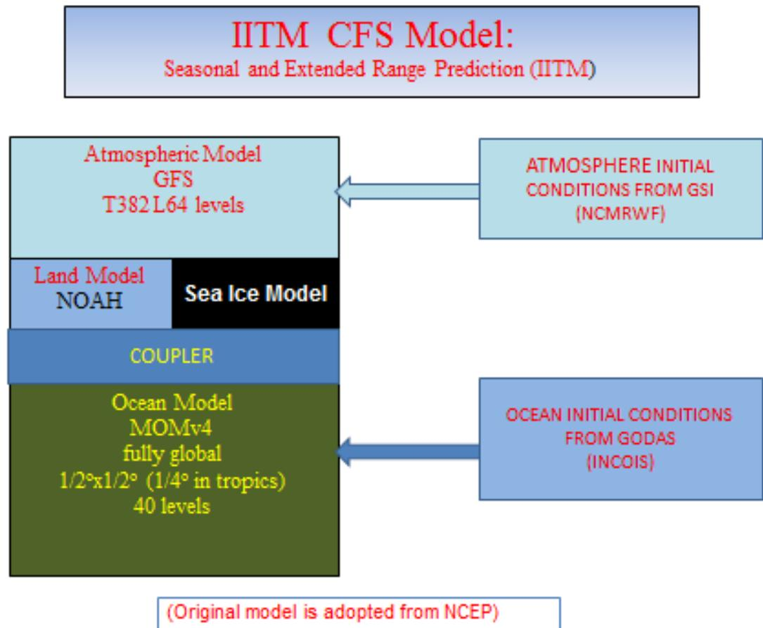
**Fig. 2:**Schematic diagram of **IITM CFS model**.
