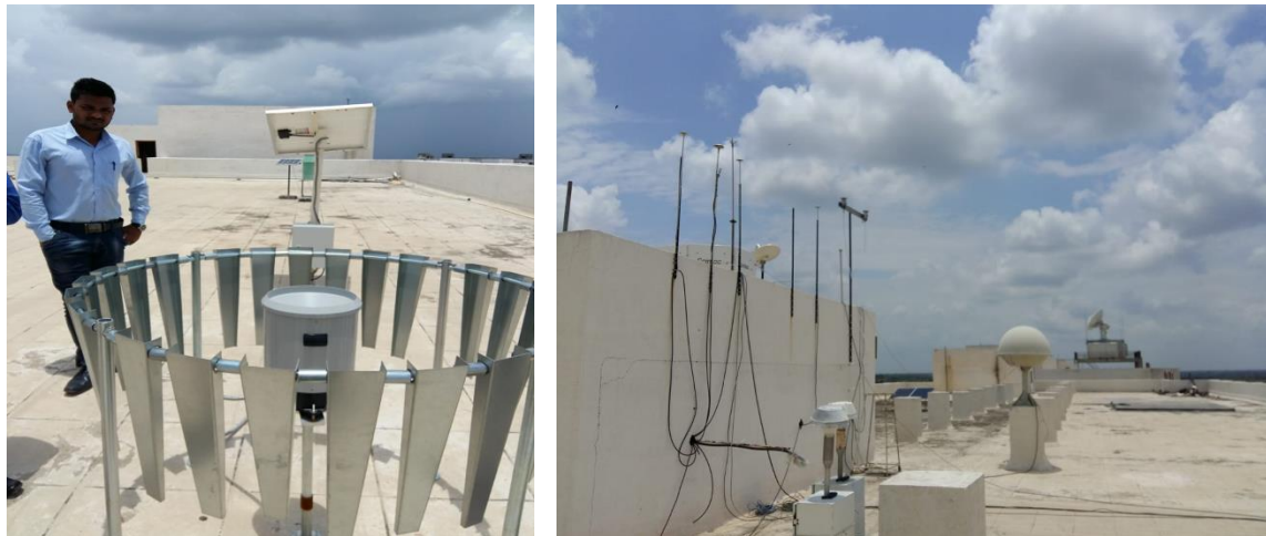
Rain gauge, Aerosol and upper air observations at NBNSCOE, Solapur
