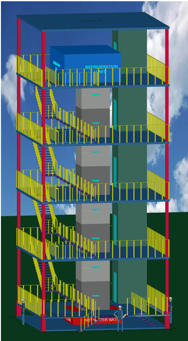
Fig. 2. Conceptual Schematic of the Fabricated Structure around the Cloud Chamber
