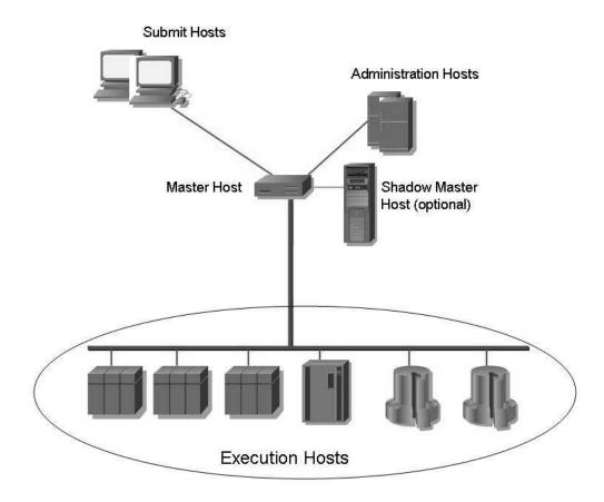
DRM monitors the host computers in the cluster for proper balancing and load conditions. Servers in a Grid / Cluster implementation are referred to as hosts. There are several types of hosts, as shown in Figure.
