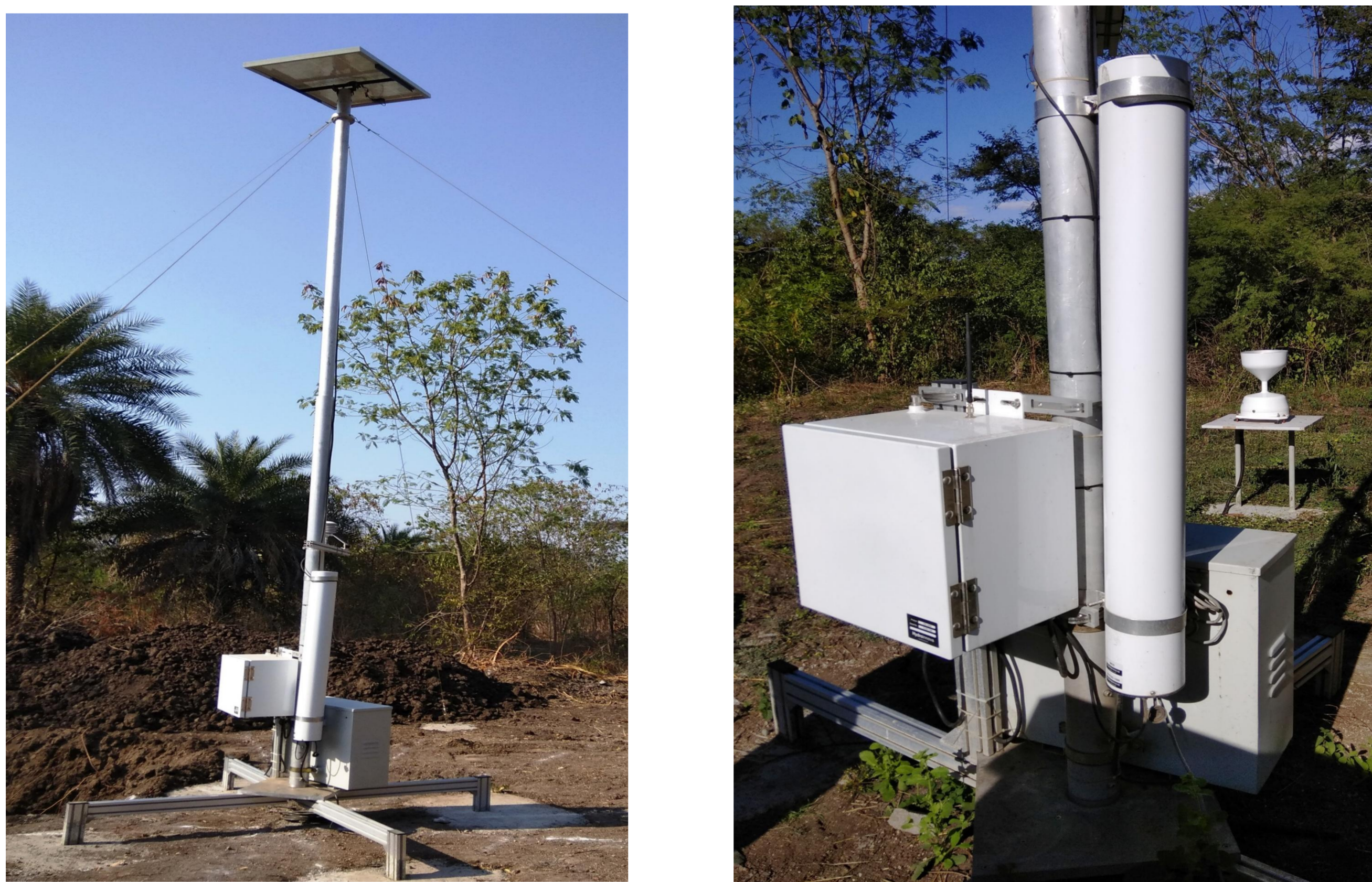
Figure 1. Cosmic-ray soil moisture sensors (CRS) installed at IITM Pune.
