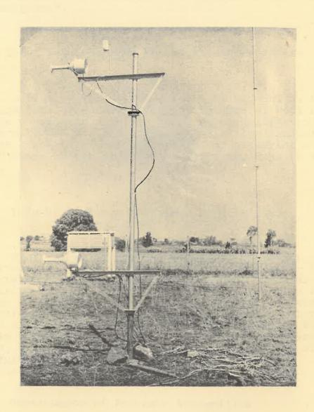
Total Solar Eclipse Observational Programme, 16 February 1980. Temperature and Humidity sensors used for the measurement of Bowen's Ratio.
