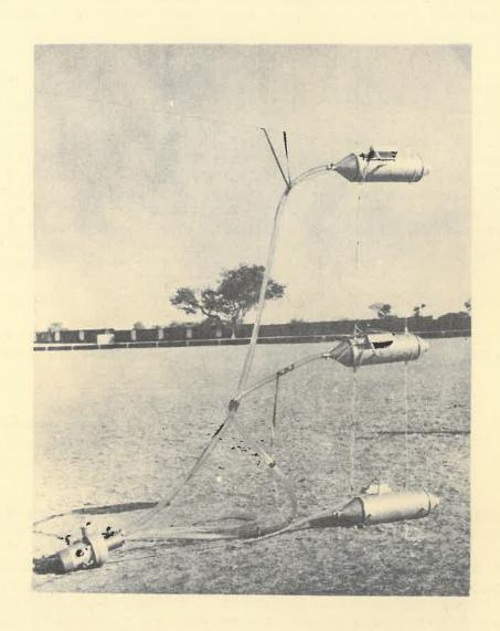
Three space charge tubes suspended in the field for the measurements of atmospheric electric space charge profiles during the solar eclipse of 16 February 1980.
