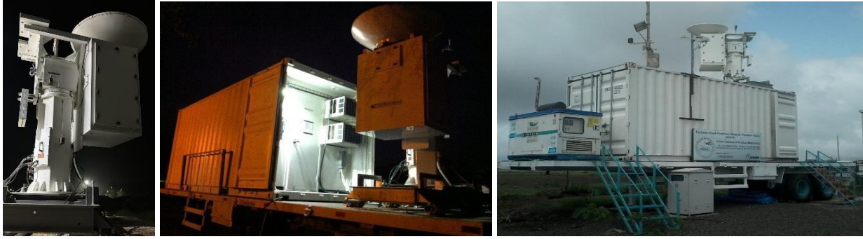
Figure 1. i. 1.2 m antenna cum RDS mount on Pedestal, 20 ft Container, and KaSPR on wheels photographs
