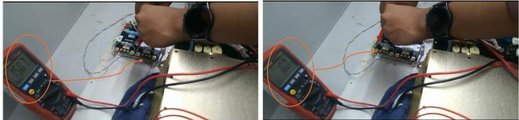
Figure 5. Isolated DC-DC converter outputs testing with DMM. The positive output power supply shows +15V, and the Negative output power supply shows 0V as marked in circles.
