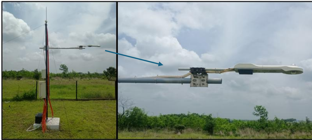
Figure 5: Net Radiometer mounted on a mast for measuring both upwelling and downwelling SW and LW radiations
