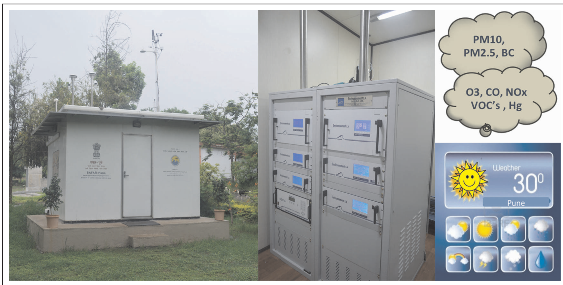
Fig. 1: Inner and outer view of SAFAR Air Quality Monitoring Station (AQMS) and Automatic Weather Station (AWS).
